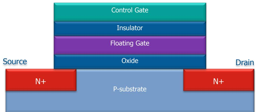
To write or clear a cell, a relative high voltage is used to force electrons to tunnel through the oxide layer to or from the floating gate. But sometimes electrons get caught in the oxide layer and contaminate the cell. This disturbs the correct readout of the cell. When this happens too much, the cell is broken. And with multiple levels in one cell, the disturbance is a problem much quicker. That's why MLC cells break so much faster than SLC cells.
